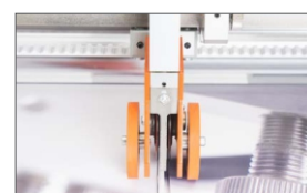
Single lengthwise rotary crush cutter (twin cutters optional)
