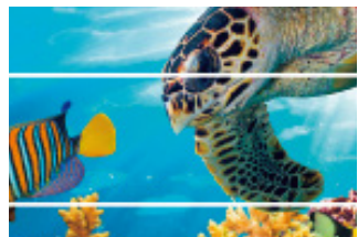
Gap/White streaks (Excessive feeding amount)
