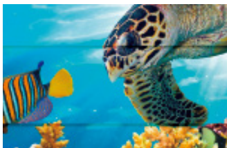
Overlap/Black streaks (Insufficient feeding amount)
