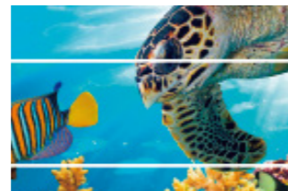
Gap/White streaks (Excessive feeding amount)
