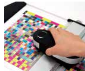
Color measurement with a colorimeter
