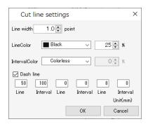
[Line Width] : Set in a range between 0.3 point and 30 point (in 0.1 point
