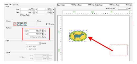
• The origin position of the job is displayed in [Width] and [Feed].
