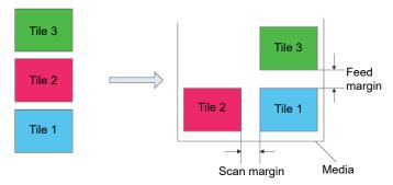
· [Sequential]: Places tiles side by side in the feed direction.
