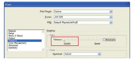
Circles and text may be printed as polygons if the scale value has not been increased in RasterLink7 or if the path output resolution has been increased in Adobe Illustrator.
