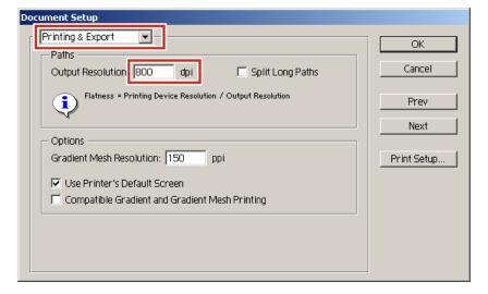
When increasing the path output resolution in Adobe Illustrator, calculate resolution using the following equation. No benefits will be gained even when a value greater than this is set.
