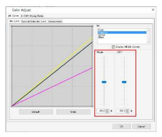
Adjust the ink limit sliders for each of the process color inks (cyan, magenta, yellow, black. etc.). [Whole] sets the ink limits for each color. [CMY] is the ink limit used when three or more inks are mixed together. The overall ink limit forms the CMY color ink limit.
