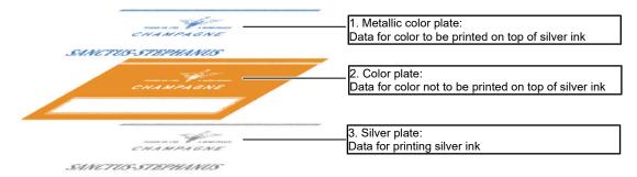
The RasterLinkTools die-cutting function allows the data for these three different plates to be created easily.
