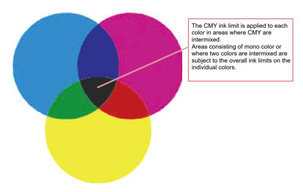
C0,M0,Y0 Using the respective overall cyan, magenta, and yellow limits C1,M1,Y1 Using the respective 3-dimensional cyan, magenta, and yellow limits
