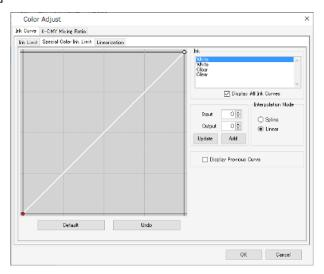
Adjust the densities for special color inks such as white, clear, and silver. Initially, the densities set in [Input] are used, but the curves should be adjusted on this screen if there is insufficient variation in the middle tone densities, such as in gradations.
