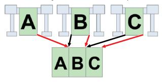
• [Reverse Even-numbered Column] selected: Tiles in even-numbered columns (tile B in this example) are rotated by 180° before printing.
