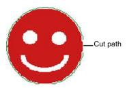
• The color of the path to be cut will be set to the spot color named "CutContour" and converted to no filling.
