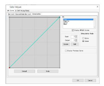
Edit the middle tone density curves for each of the process color inks (cyan, magenta, yellow, black. etc.). This adjusts the tones to ensure smooth gradations are printed for each ink.
