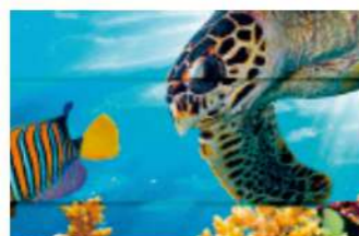
Overlap/Black streaks (Insufficient feeding amount)
